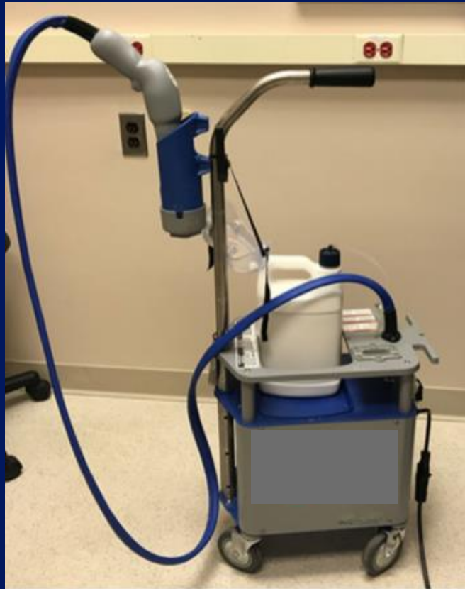
Picture of electrostatic sprayer (0.25% sodium hypochlorite)
