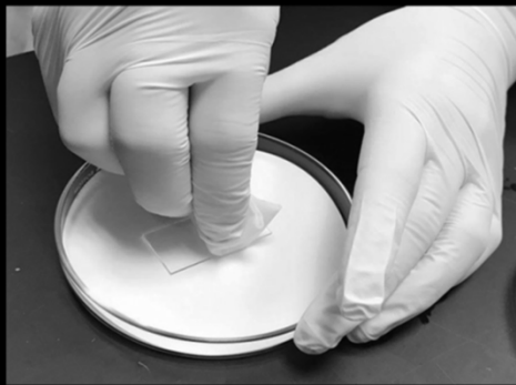
Wipe glass surface • Allow treated surface to remain undisturbed for the given contact time • The surface is not assessed for wetness
